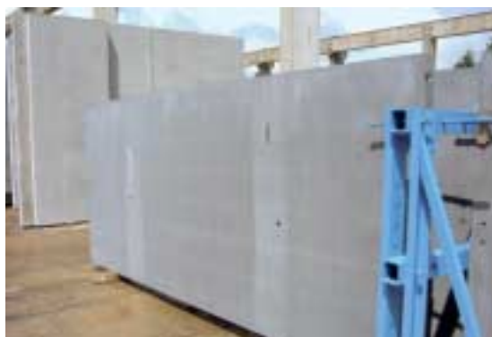
Fig. 11 The precast slabs already manufactured are stored in the yard: every component is transversely prestressed with seven strands.
