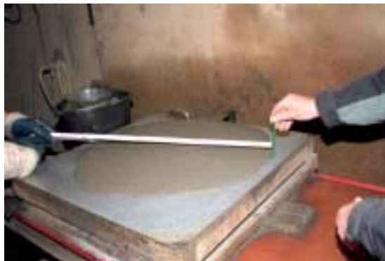
Fig. 5 Checking the spread during the mixing process.
