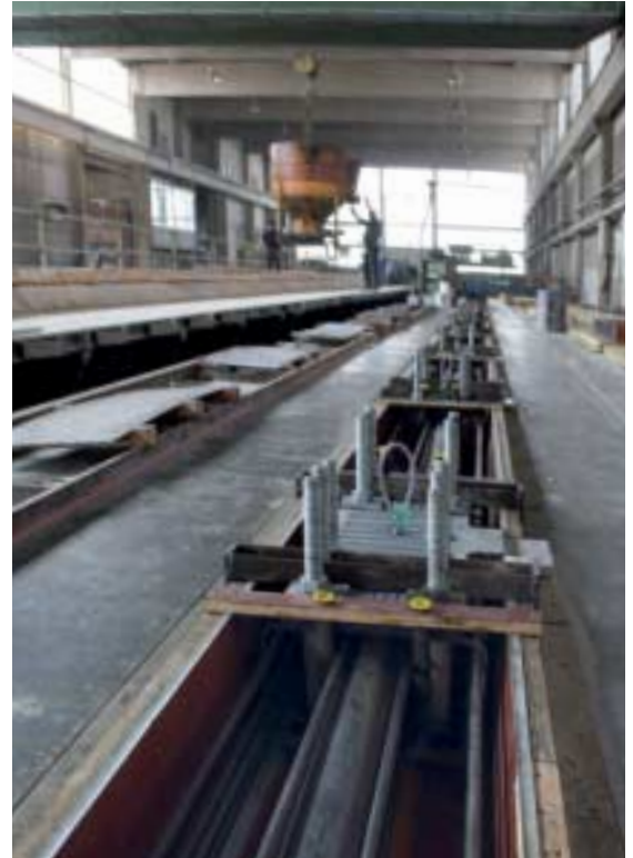
Fig. 7 The upper chords are prestressed with 10 strands. The corrugated sheath in the center of the slender girder is required for post-tensioning the individual elements after erection.
