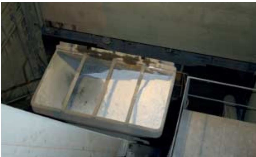
Fig. 3 Feeding the cement via the weigh unit of the mixing plant.
