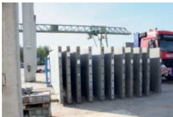
Fig. 11 The precast slabs already manufactured are stored in the yard: every component is transversely prestressed with seven strands.
